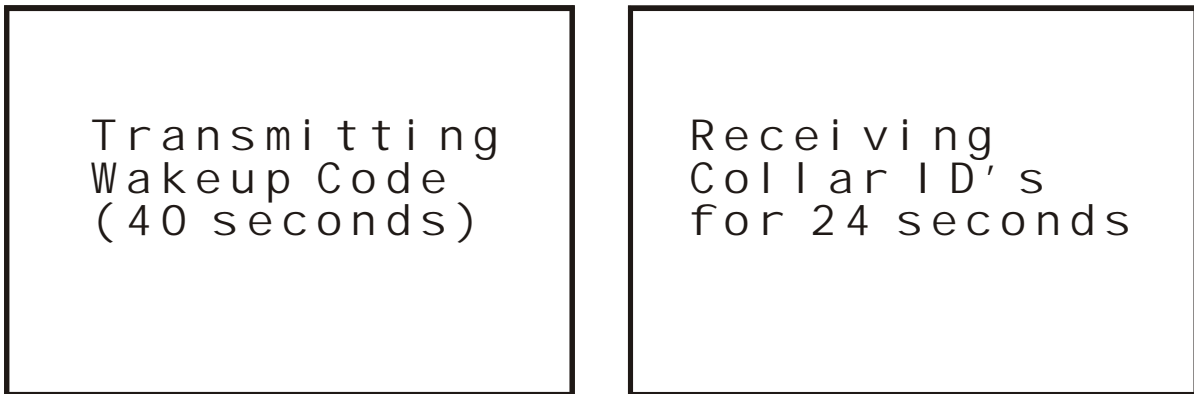
Figure 22: Display during transmitting Wakeup Code and following reception of collar ID's
