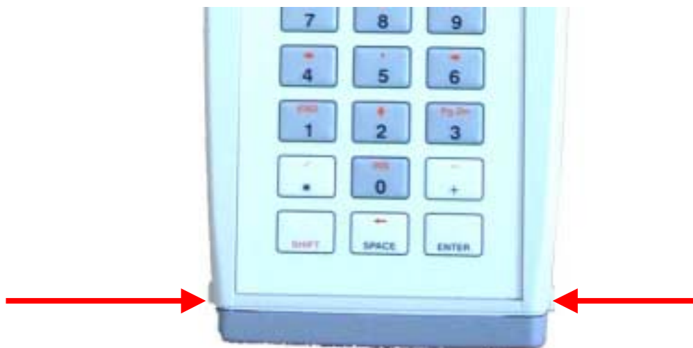
Figure 3: Location of the snap locks to remove the base cap
