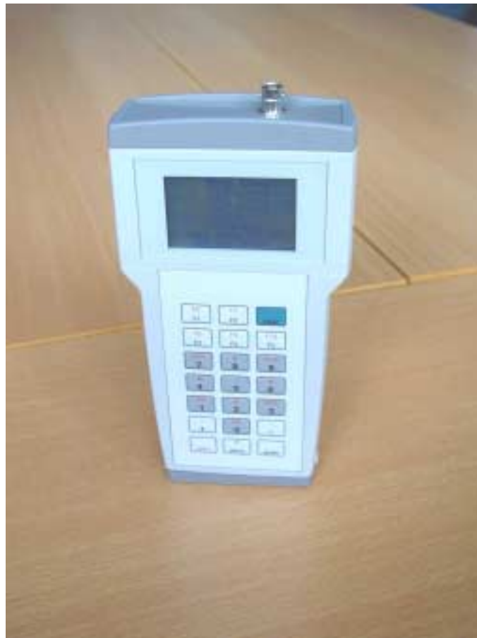
Figure 15: Place the Handheld Terminal on an iron free table during compass calibration
