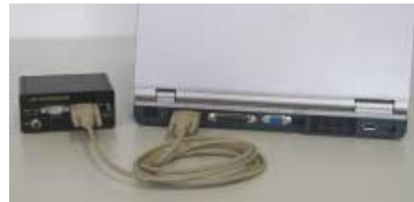
Figure 3: Connection between PC/Laptop and LM1 with a RS232 cable
