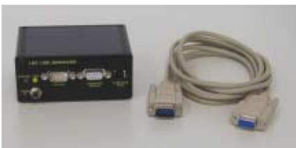
Figure 3: Connection between PC/Laptop and LM1 with a RS232 cable
